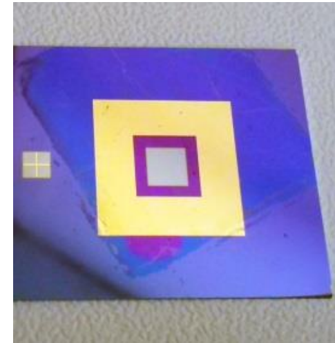
Type: n-Si, Resistivity: \rho=0.7 - 1.3 \Omega\text{cm}
